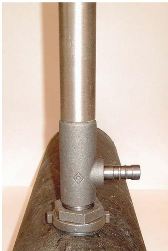
4.2 Fitting spindle and Tee assembly
