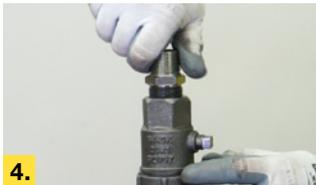
**4.** Attach the outlet Nipple to the top of the body and rotate in a clockwise direction to tighten using appropriate spanner or grips.
