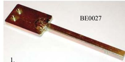
1. To open the valve, remove the closure cap and locate the key shaft into the square drive in the internal plug.
